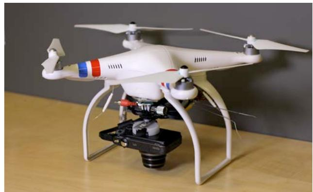
Figure 2. The DJI Phantom 2 with Canon SX260 attached.
